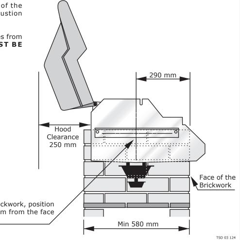
When installing BBQ head into brickwork, position the centre of "L" brackets 290 mm from the face of the brickwork.
