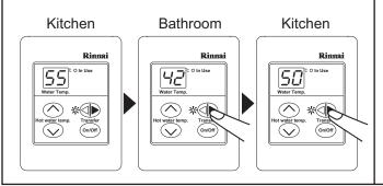
Do not push the ON/OFF button on the Kitchen Controller after having transferred priority of temperature selection to the Bathroom Controller as the system will no longer heat the water.
