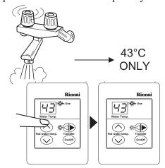
Depending on the weather conditions and the length of the pipe between the hot water unit and the tap in use, there may be a variation between the temperatures displayed at the Temperature Controller(s) and the temperature of the water at the tap.
