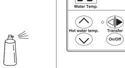
When the hot water tap is open, and hot water is flowing, the water temperature can only be increased to a maximum of 43°C on the Temperature Controller with priority.
