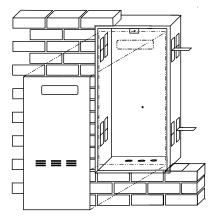
**RBOX03** this recess box is provided with a half-length front door (water heater cover is exposed). It is only suitable for semi-recessed applications.
