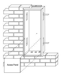
**RBOX04** this recess box is provided with a 2 front door panels (water heater cover is exposed). It is only suitable for fully-recessed applications and replaces **RBOX01**.
