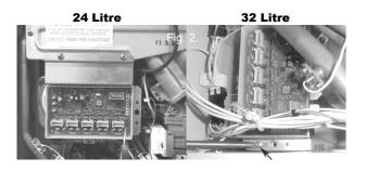
4). Connect Communication Cable B (4 wire) to socket No.1 on Master Communication PCB. (Fig. 3).
