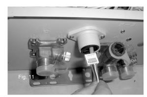
Connect Communication Cable C (unit 2) or Cable D (units 3, 4 and 5) to the 5-pin socket on the Sub Communication PCB. Connect Communication Cable A (6 pin) to the 6-pin socket on the Sub Communication PCB. (Fig 12)
