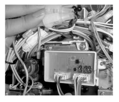
7). Connect the tail of Communication Cable A to the Infinity Main PCB as shown in Fig. 6
