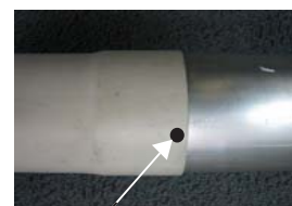
Pop rivet or 12 mm self tapping screw
